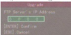
Input the ftp server IP and press **[**ENTER **]** key. DVR will connect with FTP server through network and download the firmware file.
