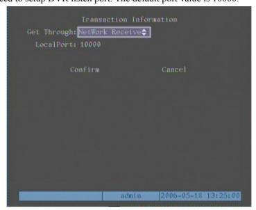
In this case, you must develop the software that is run in the ATM machine based on special protocol. The software will send the transaction information directly to the DVR. DVR will receive, analyse and overlay the text on live video.
