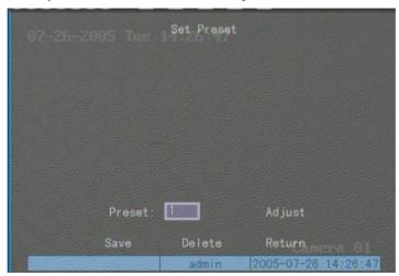
Add preset number: You can input preset number (among 1-128) in the edit box. Then press "Adjust" button to enter into PTZ control interface. In PTZ control interface, you can use direction keys to adjust PTZ position, and use [IRIS+] [IRIS-] [FOCUS+] [FOCUS-] [ZOOM+] [ZOOM-] keys to adjust iris, focus and zoom. After you finish adjusting, press [ENTER], then press "Save" button to save the preset number. You can repeat this step to setup other preset numbers.
