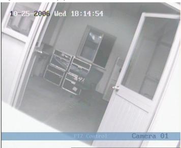
There is "PTZ Control" prompt in the PTZ control interface. The displayed camera name means which channel's PTZ is under control. For example, "Camera 01" means you are controlling the 1<sup>st</sup> camera PTZ.
